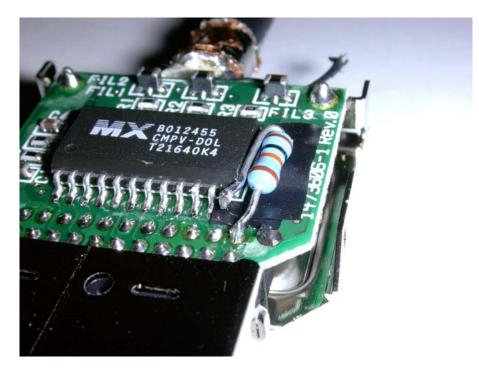
You may have noticed in the photo's above a small black wire hanging out of the back of the circuit board. Turn the board over and look near where the cable joins it, look for a small black wire soldered to the board, carefully heat the solder and pull the wire to free it.
