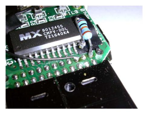
Soldering is complete, all that's left to do is to insulate the inside of the metal casing that we removed earlier, simply stick some electrical insulation tape to the corner which covers the resistor. Then carefully re-assemble the digital plug and test your cable. Here's my TV's OSD showing it's receiving an RGB image for Mr Driller (Japanese only release running on my JPN Cube).
